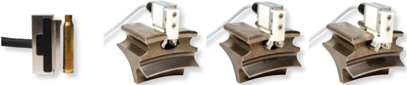
Shell inspection – This application demonstrates a single-rotation 100% inspection of small ammunition shells; the probe shown here is part of a small automated system that loads, inspects, and sentences each shell.
